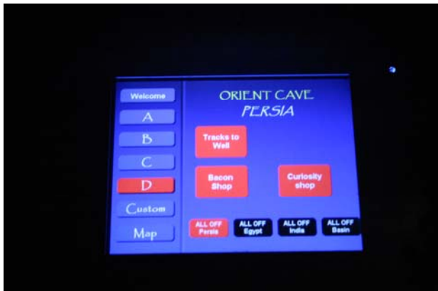
The Lighting Control Box in Orient Cave, from which every LED in the cave can be controlled, and at which guides can custom their own tours.
